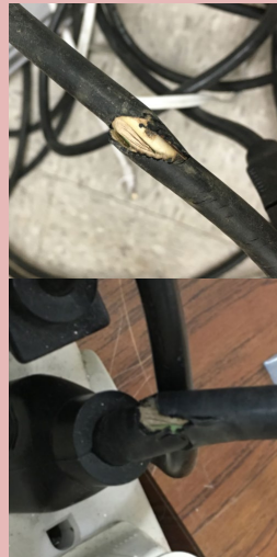
Power strip cord frayed at both ends, also daisy chained and underneath an eyewash
