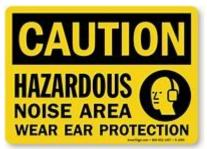
This is an example of a sign that should be posted in areas where the noise levels are at or above the 85 dBA threshold.
